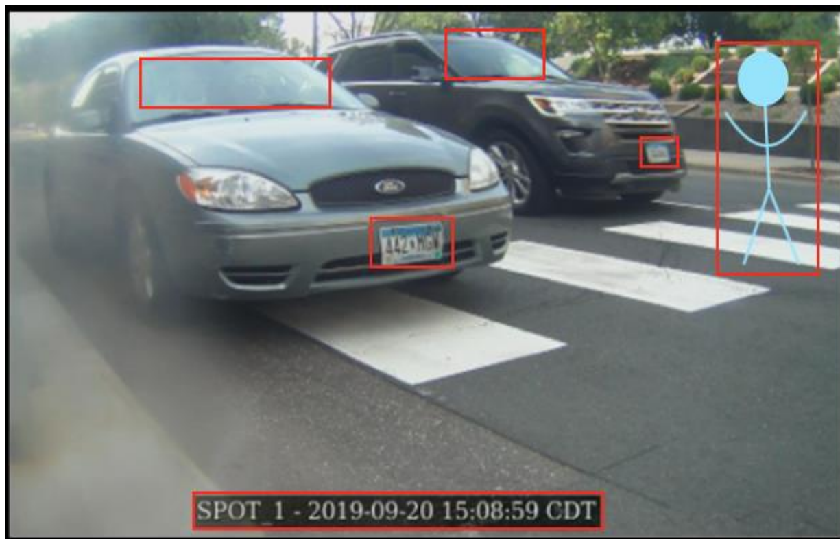
Figure 3. Still image taken from video footage of a SafetyStick (Municipal Parking Services, Inc., 2021, p. 19). Red rectangles highlight discrete data entities that may be used in the provision of parking services or by third parties for secondary uses.
